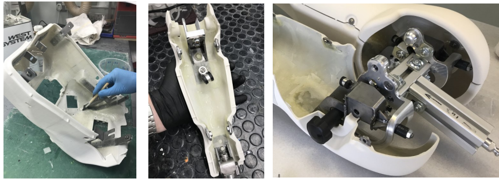
Above images: Glass fibre matting being applied inside SLS built parts alongside CNC machined, fabricated and welded components
